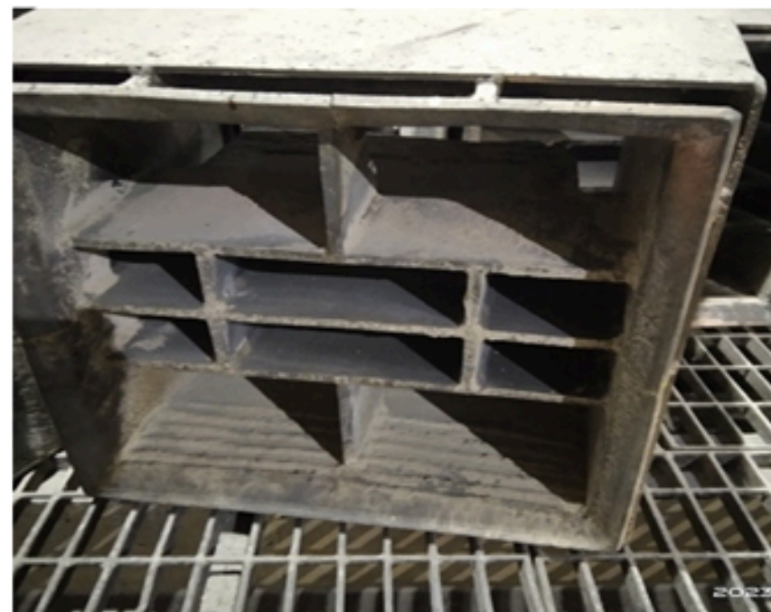
Old coal nozzle front profile
