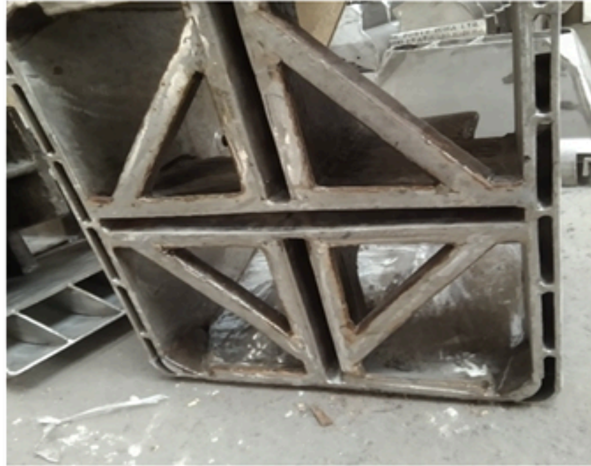
New coal nozzle front view (diamond shape)
