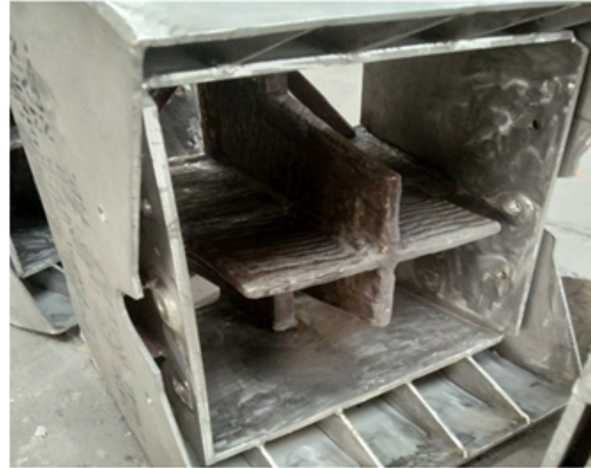
New coal nozzle rear view
